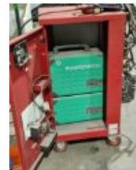
35              Migatronic Delta 160E welding machine and box of assorted welding rods.
